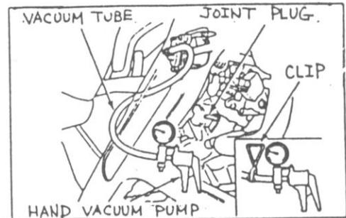
Remove the plug and the sealing washer from the front (No.2) cylinder intake port and install the vacuum gauge adapter. Connect the vacuum gauge.
