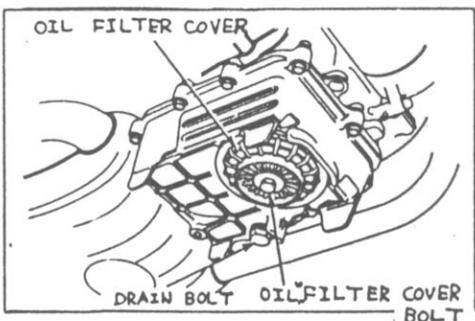
Remove the O-ring from the oil filter cover.
