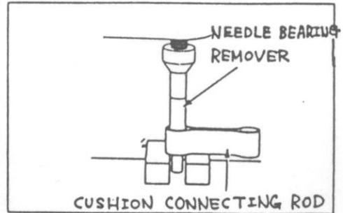
Apply grease to the cushion connecting rod needle bearing, then install the bearing into the cushion connecting rod.
