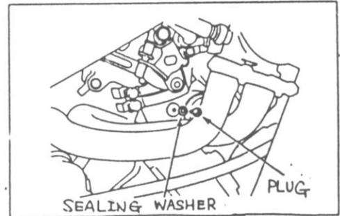
If the vacuum readings between carburetors are greater than specified, correct the difference as follows.
