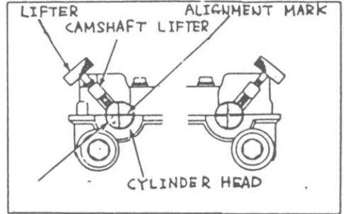
After installing the camshaft lifter, loosen the lock nut using the valve wrench, then loosen the valve adjusting screw using the valve adjust wrench.
