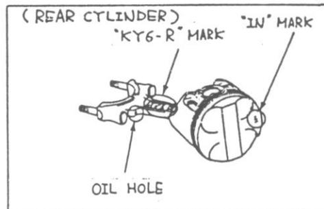
Position the piston pin and the piston pin clip into the piston groove securely.
