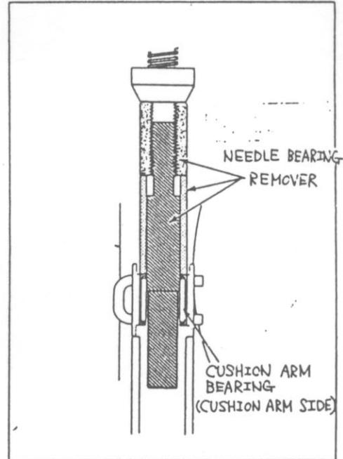
Apply grease to the new cushion arm needle bearing and install into the swingarm.
